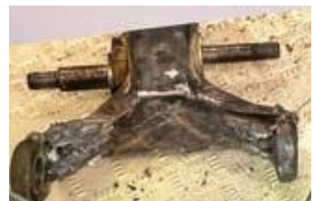
The Merlins, in their 1964 PV544, broke both wishbones, which had to be welded to get back on the road.
