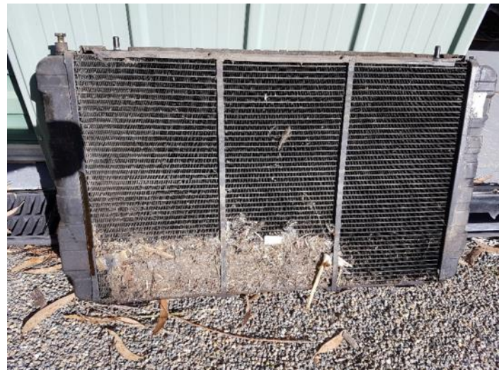
Figure 6 debris behind the oil cooler
