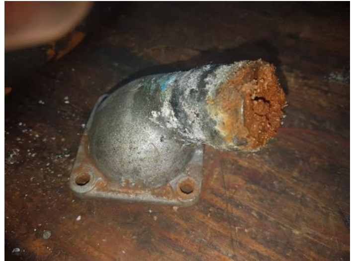
Figure 5 Buildup of corrosion in thermostat outlet
