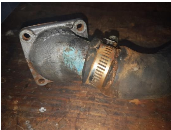
Figure 4 Split radiator hose
