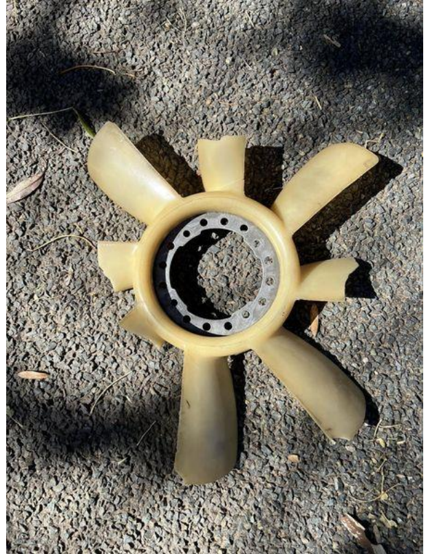
The offending cooling fan from Bruce Miller and Andrew Taurins' Capri
